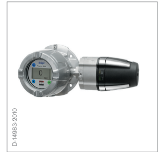
Dräger Polytron® 8720 IR Explosion-proof transmitter with optional relays and bus communication uses a high performance Dräger PIR 7200 CO2 sensor
