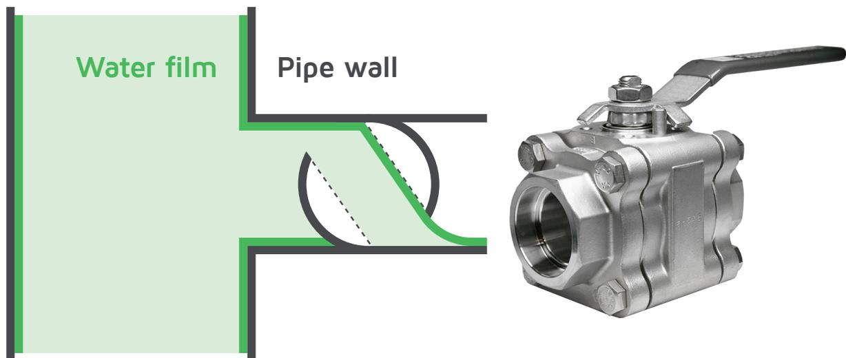
A more advanced sample valve technology is available which gives both safety and accuracy. Samplers based on an innovative piston insert design allows the pressure drop to occur inside the pipe at the valve orifice.
